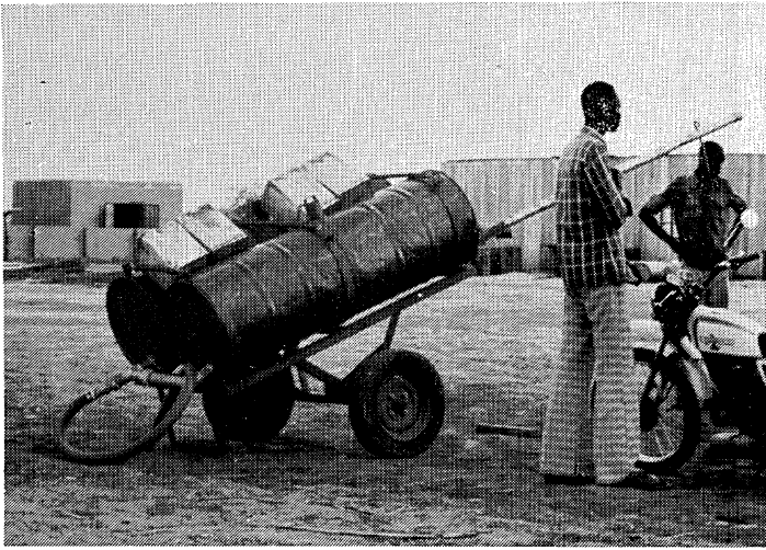
Water cart for oxen power constructed in Abyei Workshop
